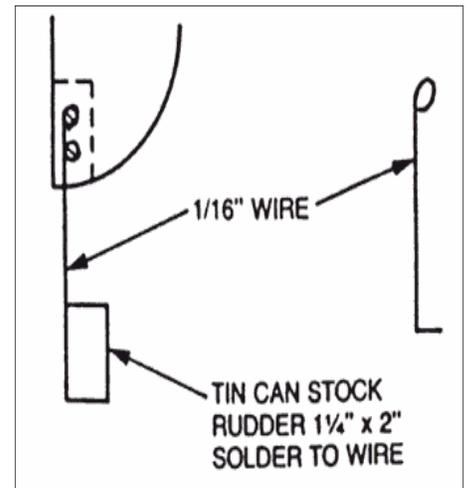
down more than 1/2" below the bottom of the end of the float. You want to make sure that at takeoff speed only the air rudder is used to steer. The water rudder is so effective that if it is in the water on a high speed run, any movement will result in a violent change of direction of the aircraft.
